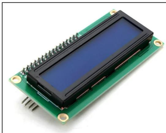
Figura 15 - Display LCD I2C.
