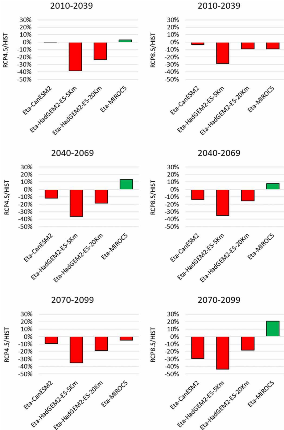
Fig. 5 | Variations in the average monthly flows of the RCP 4.5 and RCP 8.5 scenarios in relation to the historical period for each model and period. Source: by authors.
